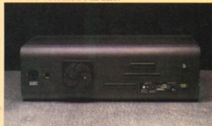
The back of the FDX shows the expansion slots and the fan inflow grill.
